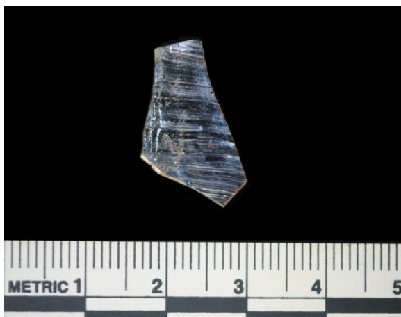
Figure 105. Colorless glass body fragment with surface texture from contact with a mold during manufacture (ER0282B).
